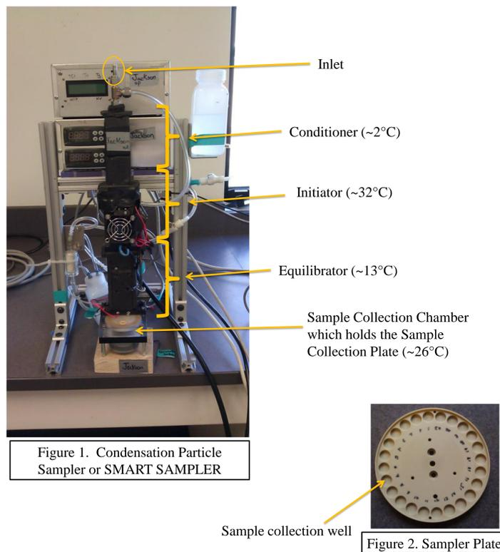
Figure 1. Condensation Particle Sampler or SMART SAMPLER
